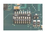
Figure 64: DIP Switch on System Unit
