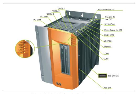
Figure 8: APC620, 5 PCI slot variant interface overview (top)
