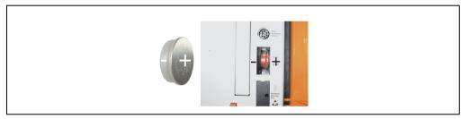
Figure 122: Battery polarity
