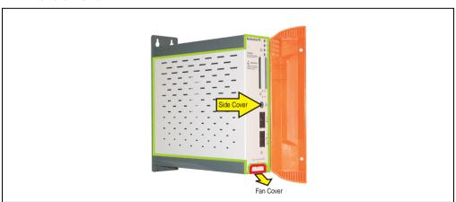
Figure 124: APC620 1PCI Slot - Remove side cover and fan kit cover
