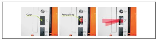
Figure 120: Battery removal
