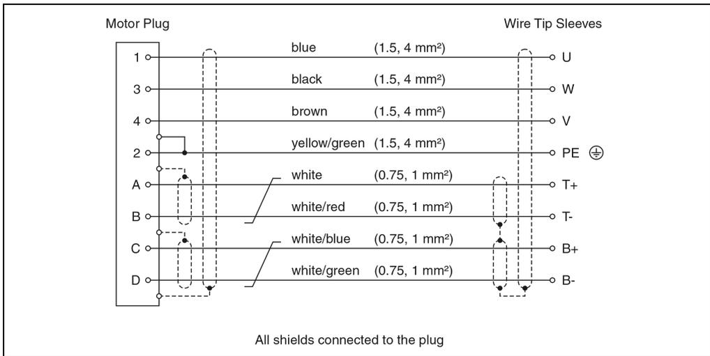
Figure 27: Cable schematic for motor cable 8CMxxx.12-1, 8CMxxx.12-3
