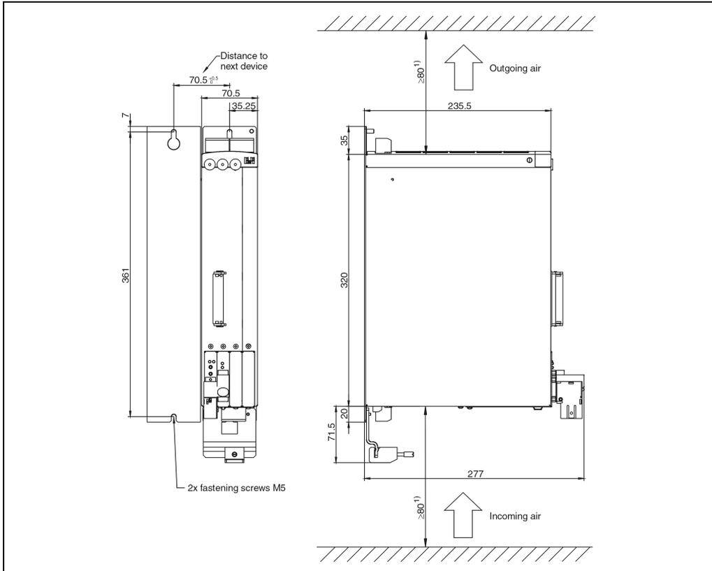
Figure 10: Dimensional diagram and installation dimensions for ACOPOS 1022, 1045, 1090
