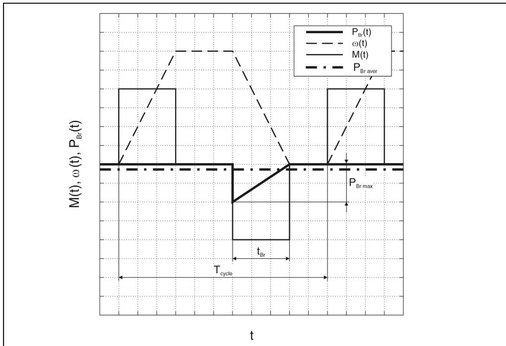
Figure 22: Diagram of a typical movement with the brake power curve  $P_{Br}(t)$  <sup>1)</sup>
