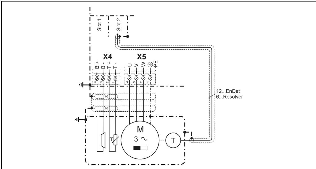
Figure 20: ACOPOS X4/X5 circuit diagram, motor connection
