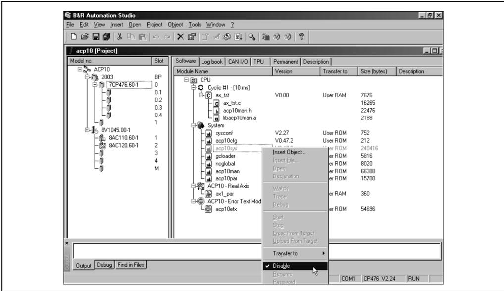
Figure 44: Enable transferring the ACOPOS operating system
