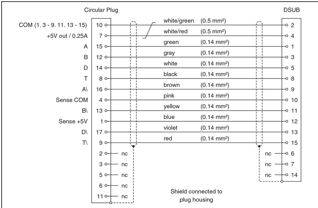
Figure 29: Cable schematic for EnDat encoder cables
