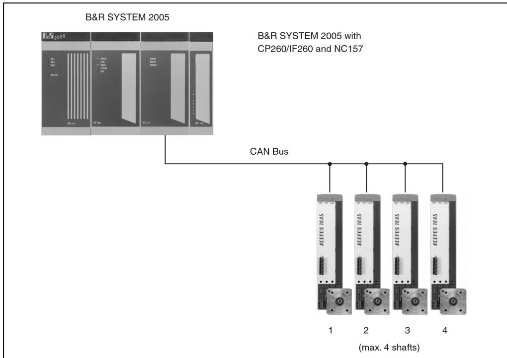
Figure 8: CAN Configuration 2
