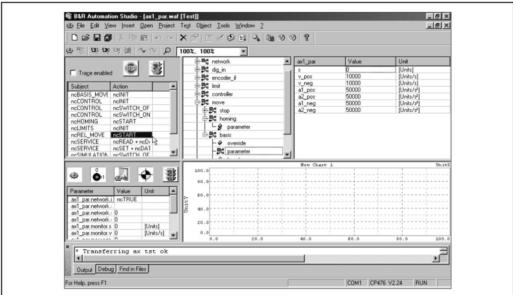
Figure 64: Test window for ACOPOS servo drives
