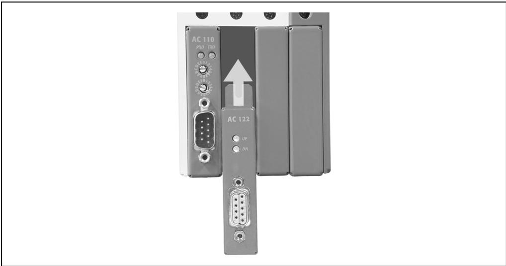
Figure 13: Installing ACOPOS plug-in modules
