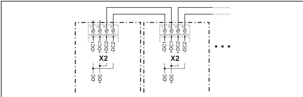
Figure 19: ACOPOS X2 circuit diagram, DC bus connections
