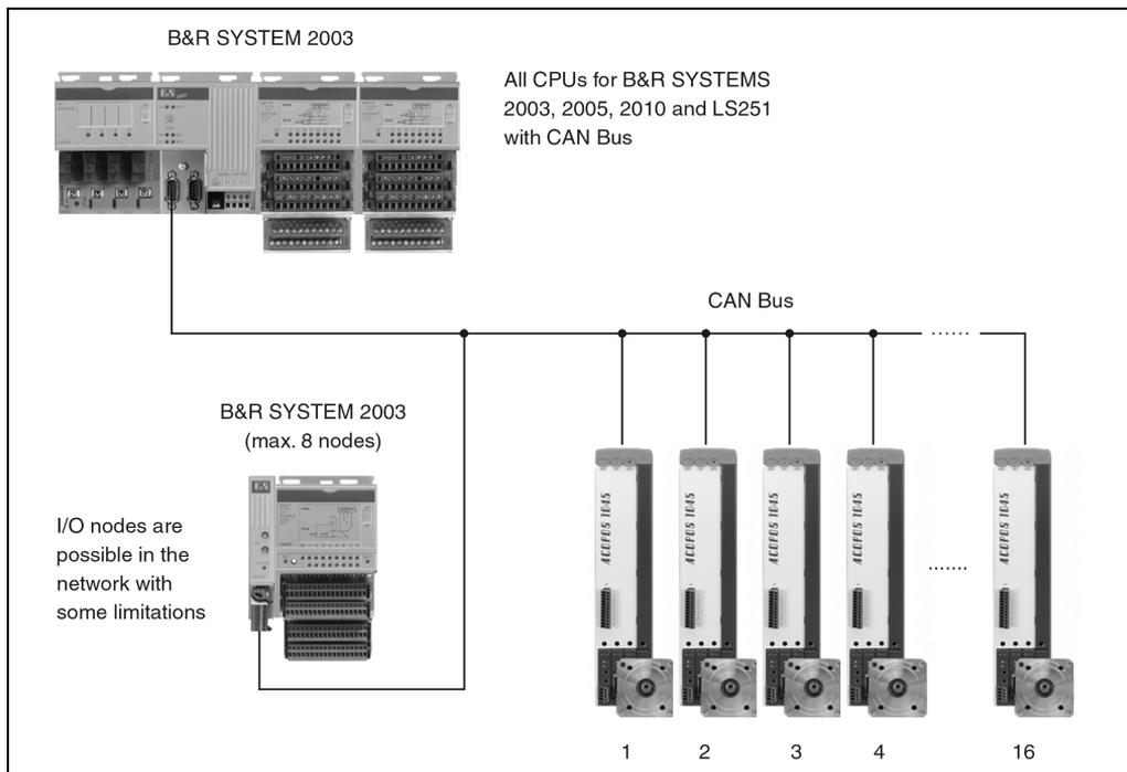
Figure 7: CAN Configuration 1
