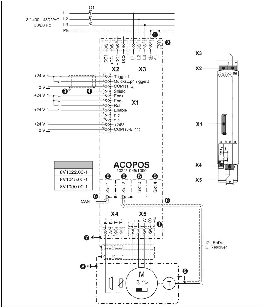
Figure 23: Connection diagram for ground and shield connections
