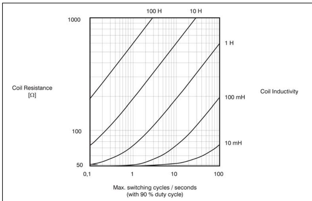
Figure 3: DO138 switching inductive loads
