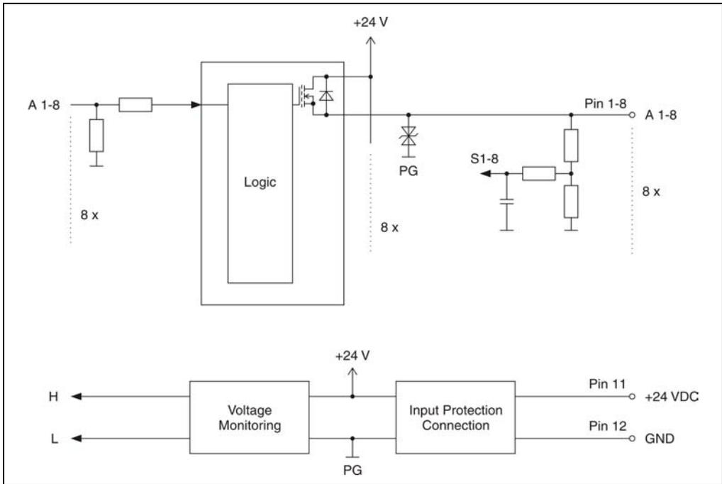
Figure 2: DO138 output circuit diagram
