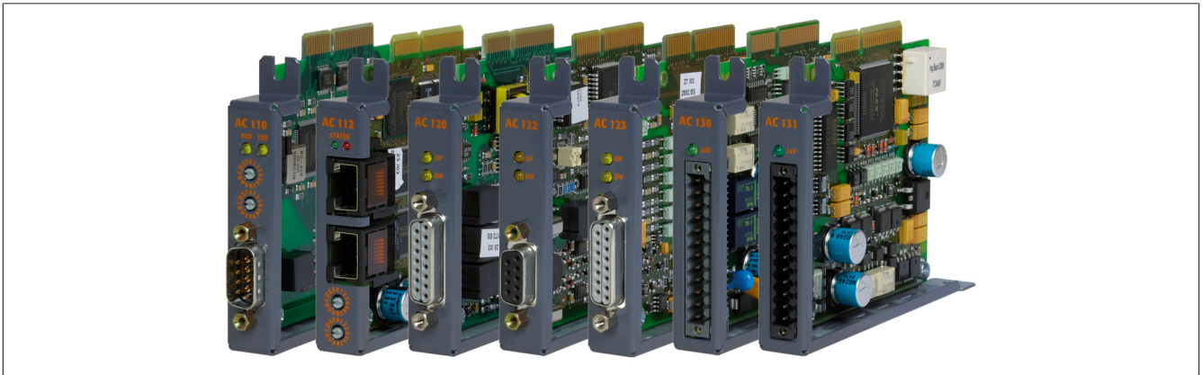
Figure 2: Plug-in modules allow optimized, application-specific configuration of ACOPOS servo drives
